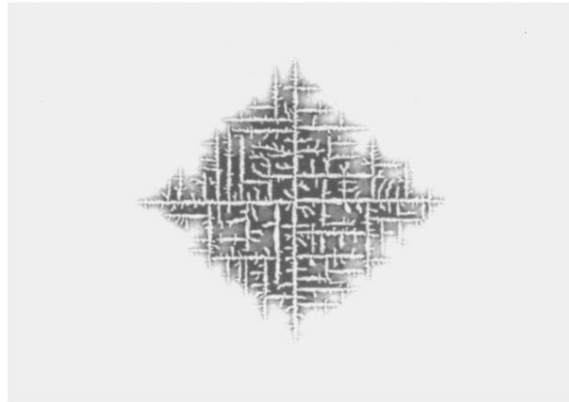
FIG. 1. Dendritic crystal grown with the lattice model. Grey levels represent temperature value of the diffusion field. Parameters are D=4.0 , m=5 , \lambda=0.015 , l_a=1 , \Delta=0.195 , and \delta=0.1 .
