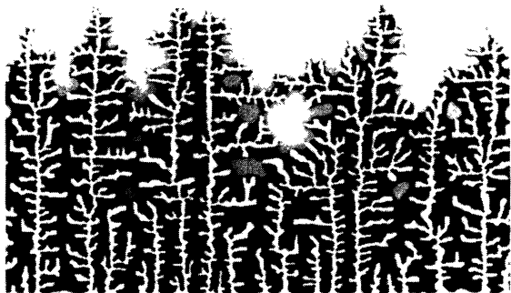
FIG. 7. Sample morphology of the growth from a planar interface. \Delta=0.1625 , \lambda=0.01 , and \delta=0.2 . Periodic boundary conditions are used in the horizontal direction.
