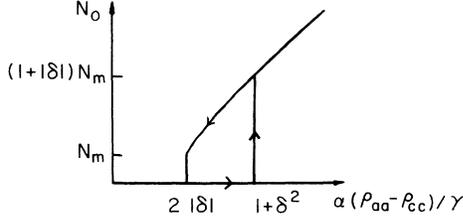
FIG. 3. Hysteresis in the two-photon laser. That  $\alpha(\rho_{aa}-\rho_{cc})/\gamma=2|\delta|$  corresponds to  $G_{\max}=\gamma$  and  $\alpha(\rho_{aa}-\rho_{cc})/\gamma=1+\delta^2$  to  $G(0)=\gamma$ .
