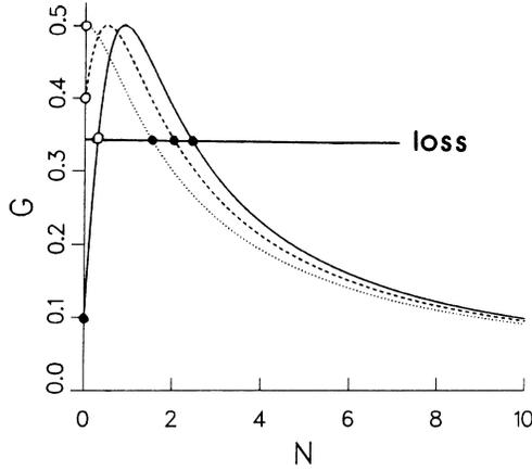
FIG. 2. Gain curve  $G$  [in units of  $\alpha(\rho_{aa} - \rho_{cc})|\delta|^{-1}$ ] of the two-photon laser as a function of a normalized laser intensity  $N = I\beta/2\alpha|\delta|$  for  $|\delta|=10$  (solid line),  $|\delta|=2$  (dashed line), and  $|\delta|=1$  (dotted line). The closed (open) circles denote stable (unstable) solutions to Eq. (4.5a).
