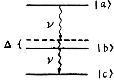
FIG. 1. Energy-level diagram for a single-mode two-photon laser.
