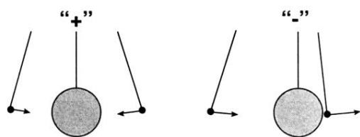
FIG. 3. "Newton's cradle" model of two-electron resonances.
