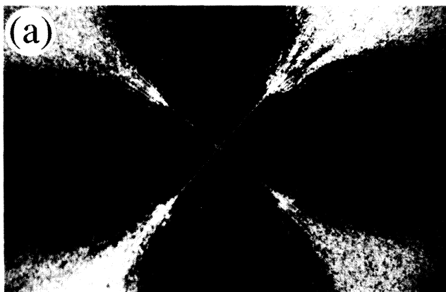
FIG. 5. Same as Fig. 4 for a [001] silicon surface inducing tilted anchoring directions (surface number 3 in Table I). One of the walls separating the domains with different anchoring directions is a solid line, which is characteristic of a tilted anchoring.
