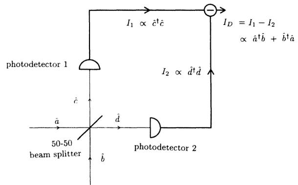
FIG. 1. Schematic of a balanced homodyne detector. The signal and local oscillator combine at a 50-50 beam splitter to give the sum and difference amplitudes  $\hat{c} = (\hat{a} + \hat{b})/\sqrt{2}$  and  $\hat{d} = (\hat{a} - \hat{b})/\sqrt{2}$ , respectively. The detector's output is given by the difference photocurrent between the two detectors—which are assumed to have equal gains.
