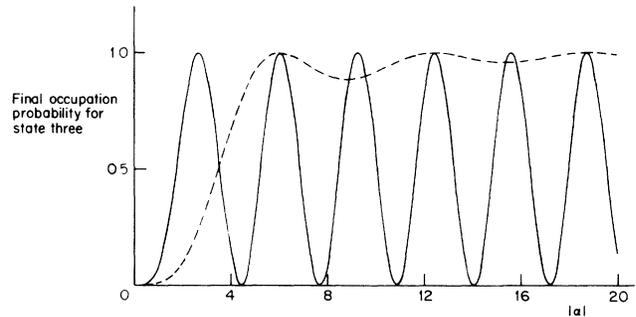
FIG. 4. Final occupation probability of state 3 plotted as a function of dimensionless amplitude for the pulses given by Eqs. (5.6)–(5.9). The solid curve is for  $\beta = \pi/2$ , and the dotted curve is for  $\beta = -\pi/2$ .
