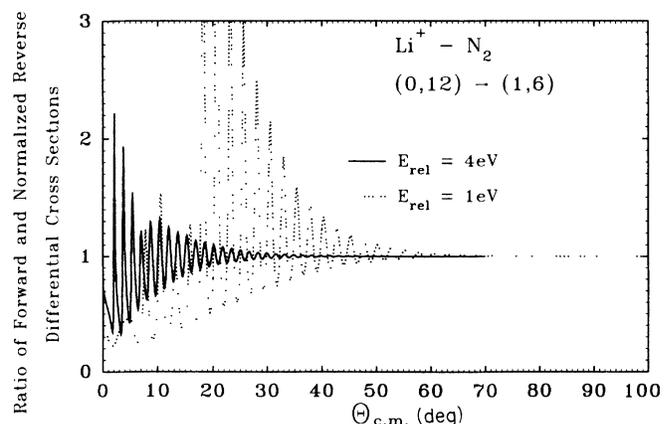
FIG. 2. Ratio of the forward and normalized reverse differential cross sections of Fig. 1 as function of center-of-mass scattering angle  $\theta^\circ$  at  $E_{\text{rel}}=1$  eV (dotted line) and  $E_{\text{rel}}=4$  eV (solid line).
