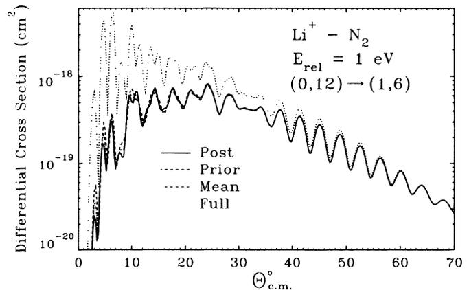
FIG. 5. Comparison of the differential cross sections for the process  $Li^+ + N_2(v=0, j=12) \rightarrow Li^+ + N_2(v'=1, j'=6)$  at relative translational energy of 4 eV for four models of  $\epsilon_s$ : post (solid line), prior (dashed line), mean (dash-dotted line), and full (dotted line).
