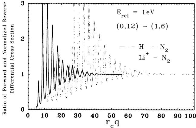
FIG. 3. Ratios of the forward and normalized reverse differential cross sections for the  $(0,12) \rightarrow (1,6)$  transitions of  $N_2$  at relative translational energy of 1 eV for collision with  $Li^+$  (dotted line) and H (solid line).
