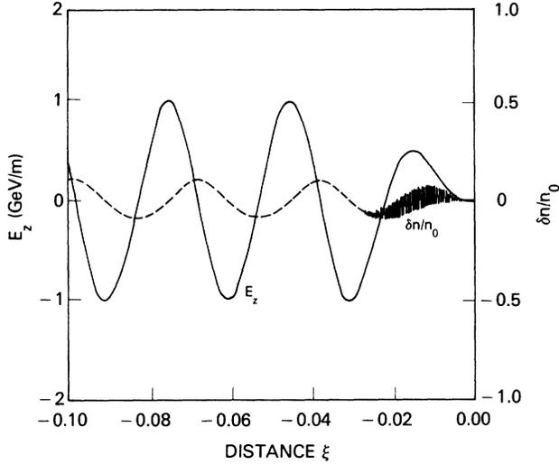
FIG. 2. Density variation  $\delta n/n_0 = n/n_0 - 1$  and axial electric field  $E_z$  in GeV/m for a laser pulse located within the region  $-L \leq \xi \leq 0$ , where  $L = \lambda_p = 0.03$  cm and  $a_{L_0} = 0.5$ .
