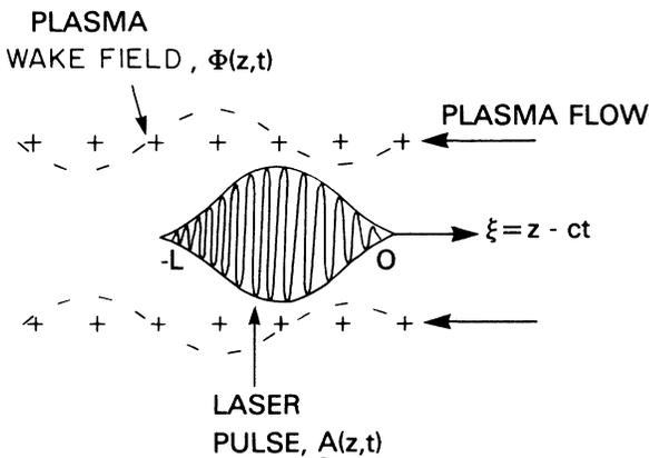
FIG. 1. Schematic showing the laser pulse in the speed of light frame ( $\xi, \tau$ ). The pulse extends from  $\xi = -L$  to  $\xi = 0$ , and the front of the pulse is at  $\xi = 0$ . In this frame the plasma flows from right to left and a quasistatic state exists.
