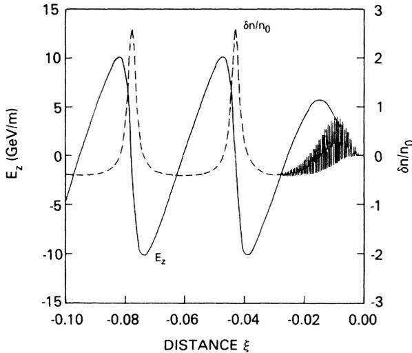
FIG. 3. Density variation  $\delta n/n_0 = n/n_0 - 1$  and axial electric field  $E_z$  in GeV/m for a laser pulse located within the region  $-L \leq \xi \leq 0$ , where  $L = \lambda_p = 0.03$  cm and  $a_{L_0} = 2.0$ .
