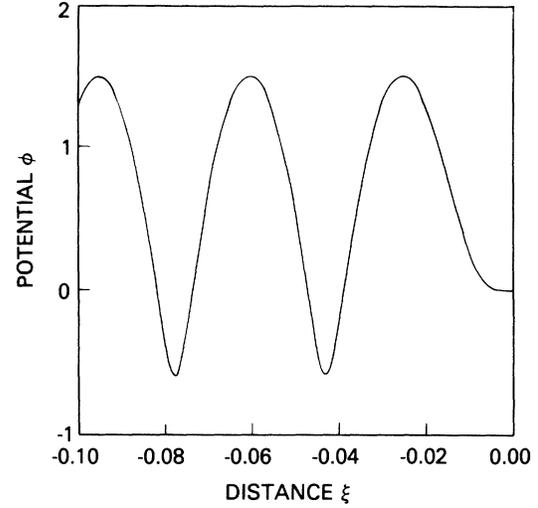
FIG. 4. Electrostatic potential  $\phi$  for a laser pulse located within the region  $-L \leq \xi \leq 0$ , where  $L = \lambda_p = 0.03$  cm and  $a_{L_0} = 2.0$ .
