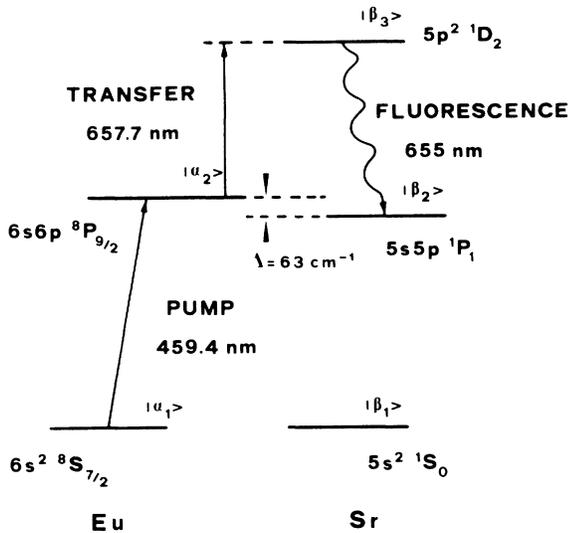
FIG. 1. Diagram of the energy levels relevant to the Eu-Sr laser-induced process. Product state basis:  $|i\rangle = |\alpha_2\rangle|\beta_1\rangle$ ;  $|x\rangle = |\alpha_1\rangle|\beta_2\rangle$ ;  $|f\rangle = |\alpha_1\rangle|\beta_3\rangle$ .
