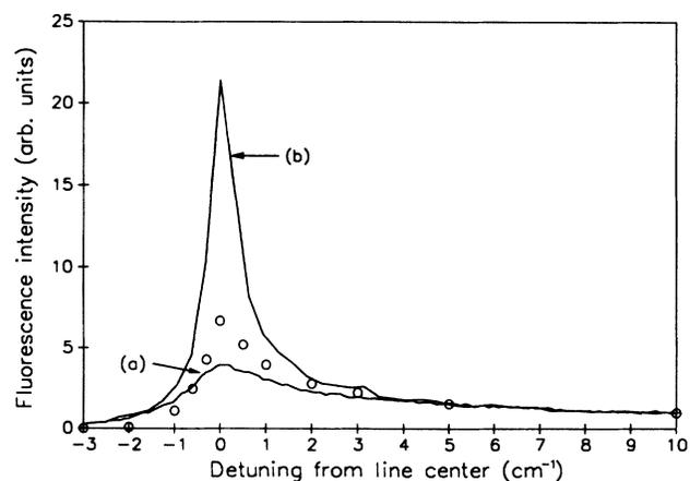
FIG. 3. Comparison between theoretical and experimental line profiles in the core region: (○) numerical results; (a) this experiment ( $90^\circ$ , fluorescence collection); (b) Ref. 14 (backward fluorescence collection).
