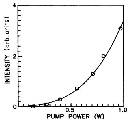
FIG. 1. Conjugate beam intensity as a function of the pump power for a suspension of PTFE microellipsoids in water. All beam polarization vectors are parallel.
