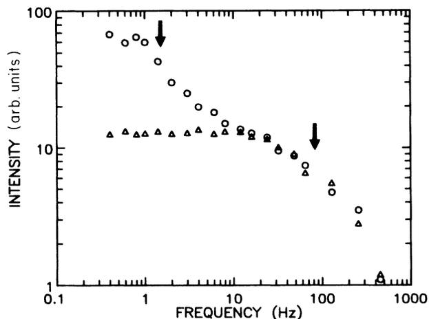
FIG. 2. Frequency response of the phase-conjugation signal for a PTFE suspension in water. Circles and triangles represent the data recorded in the  $\uparrow\uparrow\uparrow$  and in the  $\uparrow\rightarrow\uparrow$  polarization configurations, respectively (see text). The arrows in the graph indicate the cutoff frequencies.
