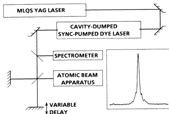
FIG. 3. The experimental apparatus is shown. The short pulse is generated by a synchronously pumped dye laser. A streak camera trace of the dye laser pulse is shown in the inset. The pulse has a width of  $25 \pm 2$  ps.
