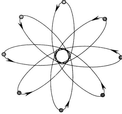
FIG. 2. An ensemble of classical states (Kepler-type orbits) is shown. The orbital motion of all the particles is in phase, i.e., their position on the orbital path is the same at a given time. The ensemble average of the motion is a shell oscillating at the Kepler orbital period.
