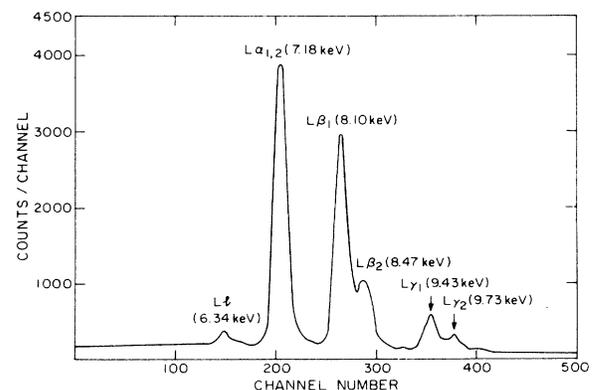
FIG. 2. Spectrum of  $L$  x rays of Tm from electron-capture decay of  $^{169}\text{Yb}$  measured with cooled Si(Li) spectrometer in random coincidence with  $K$  x rays.
