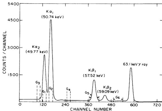
FIG. 1. Spectrum of Tm  $K$  x rays and 63.1-keV  $\gamma$  ray obtained from electron-capture decay of  $^{169}\text{Yb}$  measured with cooled Ge(HP) spectrometer in random coincidence with  $L$  x rays.  $G_1$  to  $G_6$  mark the locations of the windows set on the various parts of the spectrum as described in Sec. III A.
