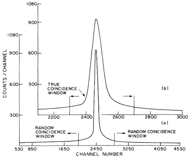
FIG. 3. Spectrum of output pulses from the time-amplitude converter. Each channel represents 0.625 nsec. (a) The true coincidence peak is shown on the background due to random coincidence events. The upper boundary of the lower 1- $\mu$ sec window and the lower boundary of the upper 1- $\mu$ sec window used to define random coincidence events are marked. (b) Enlarged portion of the spectrum showing the true coincidence peak and the 250-nsec window used to define true coincidence events.
