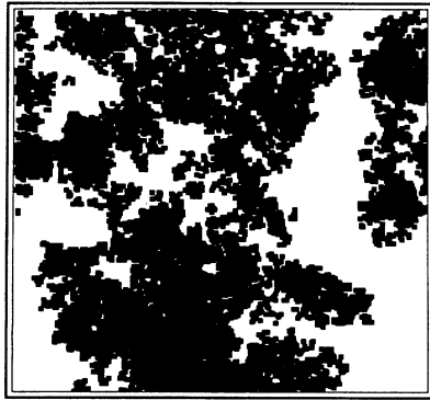
FIG. 2. Stratified percolation pattern for 5 tiers, N=7 and b=2.37 . The total area fraction occupied (colored black in the figure) is 0.64. The fractal dimension is D=1.84 . This pattern is slightly above the percolation threshold.
