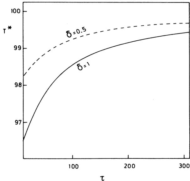
FIG. 5. Critical bifurcation time vs the correlation time of the multiplicative noise for two values of  $\delta = D/v$ .
