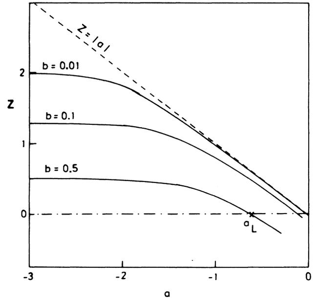
FIG. 1. Critical bifurcation parameter  $z = \mu(t^*)/\sqrt{v}$  vs  $a = \mu(0)/\sqrt{v}$  for different values of  $b = [D/x^2(0)](\pi/v)^{1/2}$ . The diagonal corresponds to  $b = 0$  and represents the deterministic case. The initial condition is deterministic and white noise is added during the sweep.
