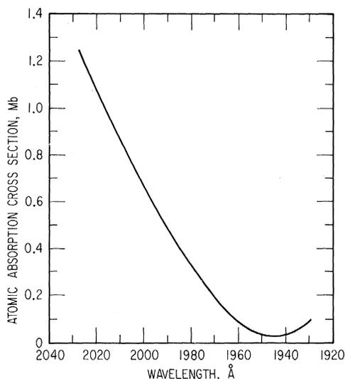
FIG. 1. Calcium continuous atomic-absorption cross section, 2028–1929 Å ( $1 \text{ Mb} = 10^{-18} \text{ cm}^2$ ).
