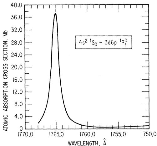
FIG. 4. Calcium atomic-absorption cross section in the vicinity of the 1765.10-Å line ( $4s^2\ ^1S_0 - 3d6p\ ^1P_1^0$ ).
