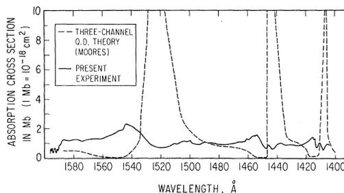
FIG. 5. Comparison of theoretical and experimental photoabsorption cross sections for calcium below 1589 Å.
