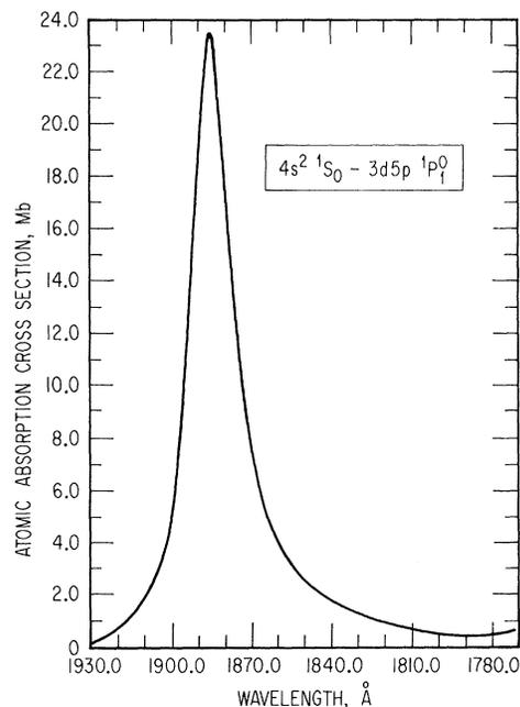
FIG. 2. Calcium atomic-absorption cross section in the vicinity of the 1885.90-Å line ( $4s^2 1S_0 - 3d5p 1P_1^0$ ).
