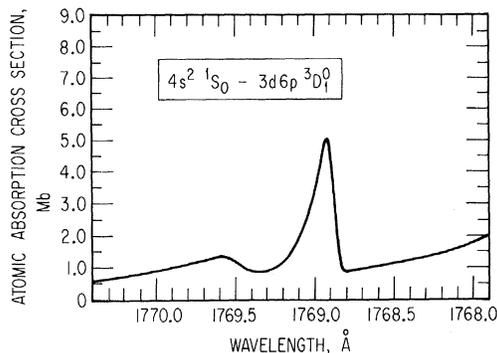
FIG. 3. Calcium atomic-absorption cross section in the vicinity of the 1768.92-Å line ( $4s^2 1S_0 - 3d6p 3D_1^0$ ).
