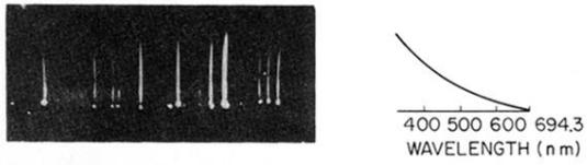
FIG. 10. Spectrum (vertical axis) vs track position (horizontal axis) of side-scattered light. A wavelength calibration curve is given to the right.
