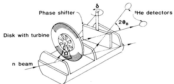
FIG. 3. Sketch of an *LLL*-type interferometer showing the placement of the aluminum disk containing the Sm foils in between the splitter and the mirror blades. The shaded segments on the disk correspond to the positions of the Sm foils. The positions of the detectors and the aluminum phase shifter are also shown.
