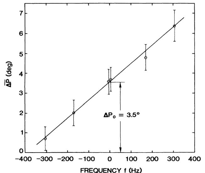
FIG. 6. A linear regression fit of the experimentally determined  $\bar{\Delta P}$  values against the disk rotation frequency  $f$ . Intercept of the linear fit on the ordinate yields  $\Delta P_0$ .
