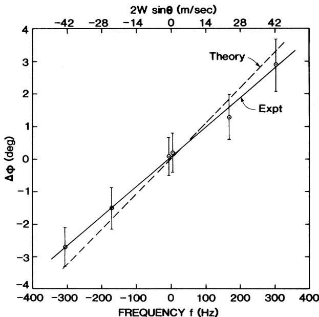
FIG. 7. Plot of experimental and calculated motion induced phase shifts  $\Delta\Phi$  against disk rotation frequency  $f$ . The velocity components of the disk motion along the beam directions, which caused these phase shifts, are listed along the top x axis.
