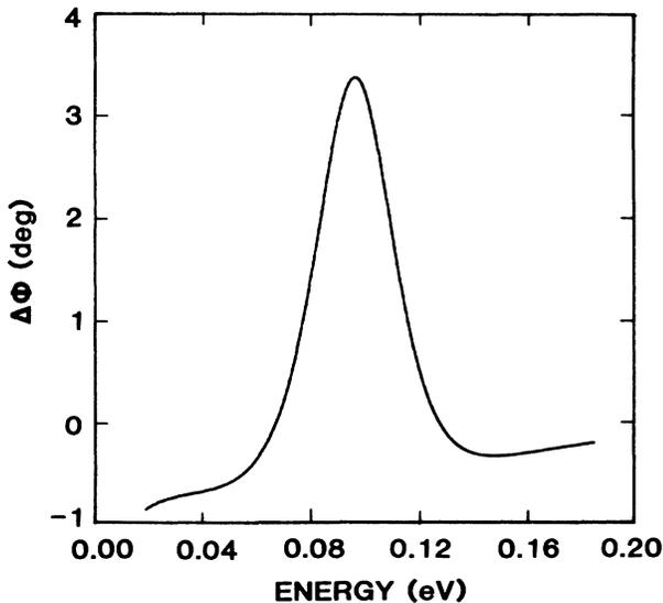
FIG. 2. Calculated phase shift of a neutron wave passing through moving natural Sm foil. In this case the foil thickness is  $33 \mu\text{m}$  and the foil velocity ( $W$ ) is approximately  $87 \text{ m/sec}$ . [See Eq. (9)].
