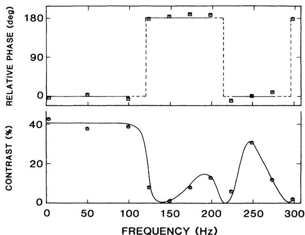
FIG. 8. Effects of transmitted vibration on the phase and contrast of interference pattern in the early version of this experiment. The magnitude of the transmitted vibration depended on the rotation frequency of the disk.
