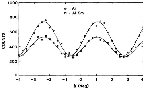
FIG. 5. Neutron interferograms of a typical run at 303 Hz rotation frequency of the disk. Data collection times for the Al and Al-Sm sectors were 2 and 6 min per point, respectively.
