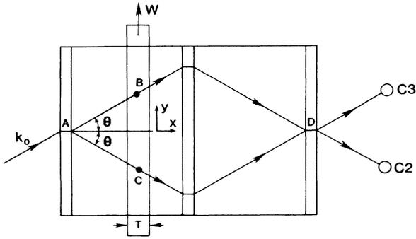
FIG. 1. Schematic of an *LLL*-type neutron interferometer showing the beam paths.
