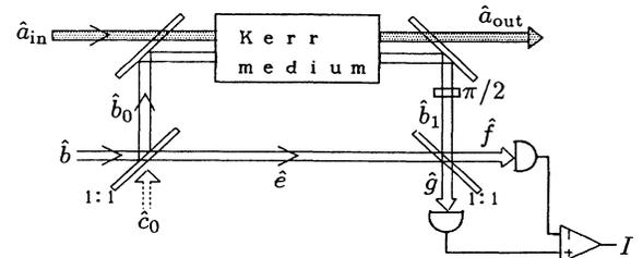
FIG. 4. Photon number QND measurement scheme with the Kerr effect under loss-free conditions (Ref. 4). The signal photon-number modulates the probe phase via the loss-free Kerr effect. The probe phase is measured by means of the Mach-Zehnder interferometer with a balanced mixer detector.
