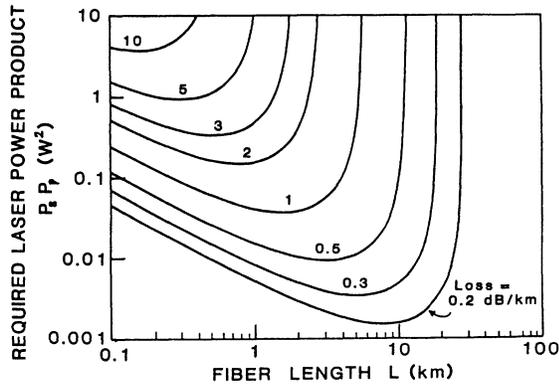
FIG. 8. Required laser power product vs medium length. A single-mode optical silica fiber is assumed as the Kerr medium. Parameters used are as follows:  $\chi^{(3)} = 3.6 \times 10^{-33}$  (MKS),  $\lambda_s = 1.55 \mu\text{m}$ ,  $\lambda_p = 1.32 \mu\text{m}$ ,  $A_{\text{eff}} = 50 \mu\text{m}^2$ , and  $n = 1.45$ .
