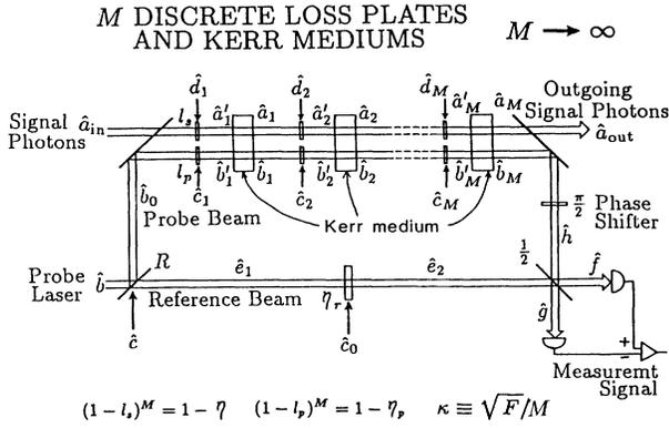
FIG. 6. Model of the QND measurement scheme with a lossy Kerr medium. Alternating loss plates and Kerr media represent a lossy Kerr medium. The number of the plates  $M$  is set to be  $\infty$  under the constraint of a constant total loss and the Kerr effect.
