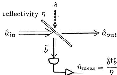
FIG. 2. A dissipative photon-number measurement with a beamsplitter and an ideal photon counting. Vacuum fluctuation  $\hat{c}$  is linearly coupled to the incident field  $\hat{a}_{\text{in}}$ .
