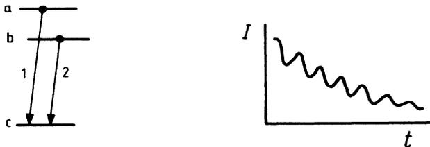
FIG. 4. Scheme for quantum-beat experiments. Coherent superposition of upper levels  $a$  and  $b$  decay to ground state  $c$ . The detector current shows a modulation in addition to the usual exponential decay.
