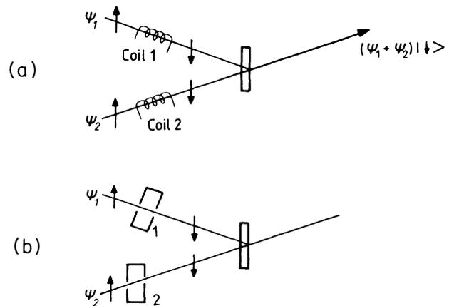
FIG. 3. (a) Neutrons from crystals  $S_1$  and  $S_2$  are passed through two coils and spin flipped from up to down. These two beams are then recombined and total wave function is found to be a coherent superposition of the two spin-down partial waves. (b) In this figure we replace the coils of (a) by micromaser cavities.
