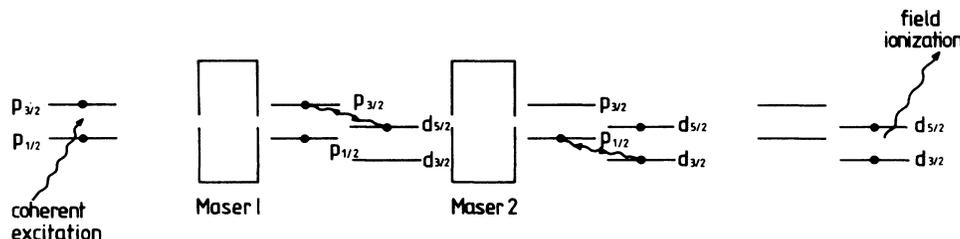
FIG. 6. Quantum-beat experiment using micromaser *Welcher Weg* detectors in which quantum beats are detected via field ionization rather than spontaneous emission.
