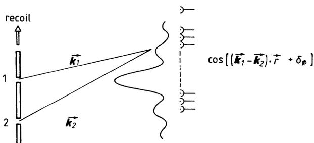
FIG. 1. Figure depicting the Einstein-Bohr recoiling-slit *Gedanken* experiment. Light emerging from slits 1 and 2 is collected by an array of photodetectors displaying the usual Young’s double-slit interference pattern.
