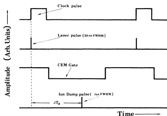
FIG. 2. Ion-trap and laser timing diagram. The channel electron multiplier (CEM) is gated off during laser ablation to avoid damage to it from the large number of laser-induced ions. The ion dump pulse is used to allow stored ions to exit the trap and move toward the CEM. The ion dump pulse is delayed relative to the ablation event  $\Delta T_d$  ranging from 20 ms to 2 s.
