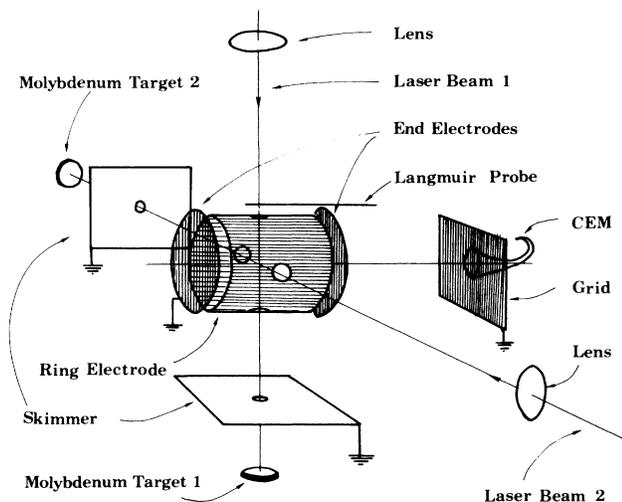
FIG. 1. Laser ablation and ion-trap apparatus.
