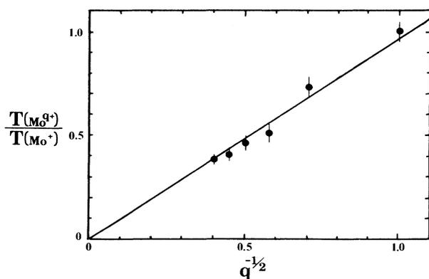
FIG. 5. Ions time of flight and charge-state identification. Shown plotted are measured times of flight normalized to the time of flight for  $Mo^+$  vs the charge state  $q^{-1/2}$ . The data fit a straight line with a slope of  $0.97 \pm 0.09$ , clearly indicating a correct charge-state identification.  $q_z$  and  $a_z$  are the parameters used in the Mathieu equation (Refs. 12 and 13).
