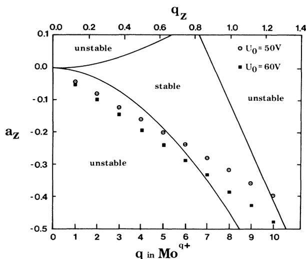
FIG. 4. Ion stability diagram for molybdenum. The ion trap with  $r_0=1.63$  cm,  $z_0=1.68$  cm is operated at  $V_0=315$  V,  $f=0.8$  MHz. Ions in the region labeled "stable" can be stored in the trap. The dc voltage  $U_0$  on the ring electrode selects which ions are stored. Increasing  $U_0$  from 50 to 60 V shifts  $\text{Mo}^{6+}$  out of the stable region. An ion signal is observed at  $U_0=50$  V but not at  $U_0=60$  V.
