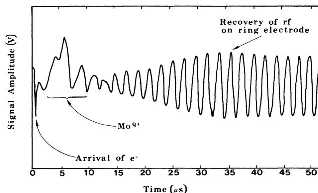
FIG. 7. Langmuir probe signal. The arrival of electrons and ions at the trap is detected almost immediately after ablation indicating that the ions' energies must be near 250 eV. Note that the probe also picks up a rf signal from the ring electrode. The presence of the electrons and ions from the ablation pulse influence greatly the rf amplitude at the ring electrode, effectively shorting it out momentarily.
