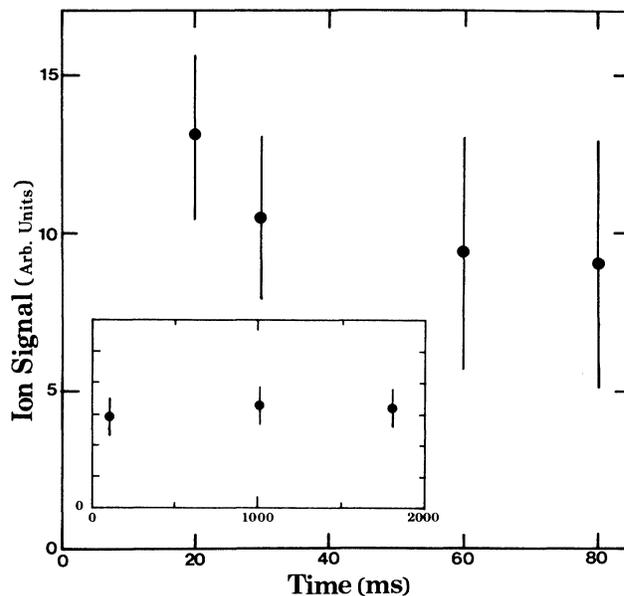
FIG. 6.  $W^{4+}$  signal amplitude as a function of storage time. The storage time is in excess of 2 s. The main figure shows the ion signal over a period of 80 ms, while the inset shows ion signal essentially constant to 2 s. The initial decay of the ion signal may be due to enhanced background gas pressure following laser ablation.
