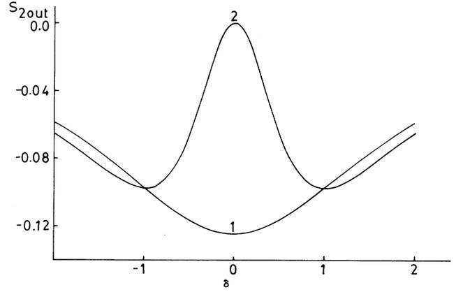
FIG. 7. Squeezing spectrum  $S_{2out}(\delta)$  of the output as a function of  $\delta$  for no atom in the cavity ( $g=0$ , curve 1) and for an atom in the cavity ( $g=1$ , curve 2). The parameters are  $\Gamma=\nu=0, \kappa=1, |G|=0.9$ .
