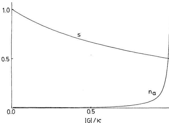
FIG. 1. Mean excitation  $n_a$  and the squeezing parameter  $s$  [Eq. (3.11)] for the oscillator as a function of  $|G|/\kappa$  for  $\Gamma = \nu = 0$ . Each curve is normalized to its maximum value.
