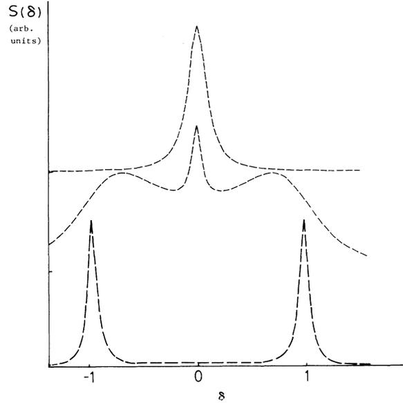
FIG. 2. Fluctuation spectrum  $S(\delta)$  as a function of  $\delta$  for  $\kappa = 10, g = 1, \Gamma = \nu = 0$  and for  $|G| = 0, 9$ , and  $9.9$  (top to bottom). For clarity different curves are displaced. Each curve is normalized to its maximum value. The starting point on the  $y$  axis for each curve is marked.
