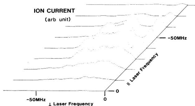
FIG. 2. Ion current vs laser detunings to measure the capture range of the trap.
