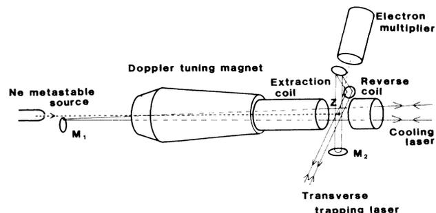
FIG. 1. Experimental configuration. Z is the zero magnetic-field point, and  $M_1$  and  $M_2$  are the polarization reversing mirrors consisting of a  $\frac{1}{4}$  wave plate with 100% reflection coating on the backside.
