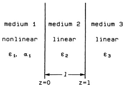
FIG. 4. Schematic of the layered guiding structure. For the thin-metal-film case  $\epsilon_3 > \epsilon_1 > 0$ ,  $\epsilon_2 < 0$  and for the dielectric-layer case  $\epsilon_2 > \{\epsilon_1, \epsilon_3\} > 0$ .
