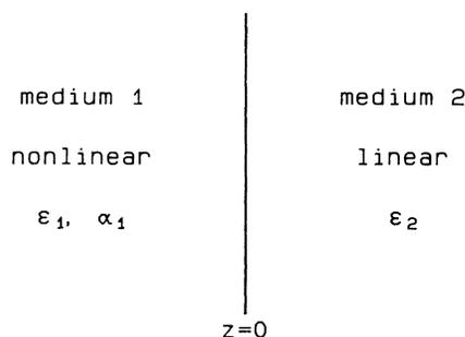
FIG. 2. Schematic of single-interface guiding structure:  $\epsilon_2 > \epsilon_1 > 0$ ,  $\alpha_1 > 0$ .
