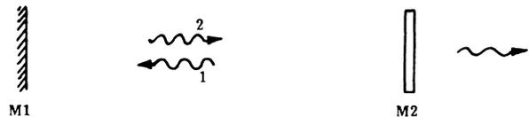
FIG. 1. A schematic diagram of a laser cavity with the two traveling-wave modes denoted by 1 and 2. Mirror  $M1$  is assumed to be perfectly reflecting, while the output mirror  $M2$  is partially transmitting. The complex reflection coefficients of their inner surfaces are  $e^{i\phi_1}$  and  $\rho e^{i\phi_2}$ , respectively.
