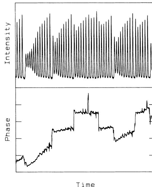
FIG. 2. Intensity and phase for the FIR ammonia laser studied in Ref. 1. The operating parameters correspond approximately to those used in Figs. 1(c) and 1(d). The vertical axis for the phase has tick marks every  $\pi$ .
