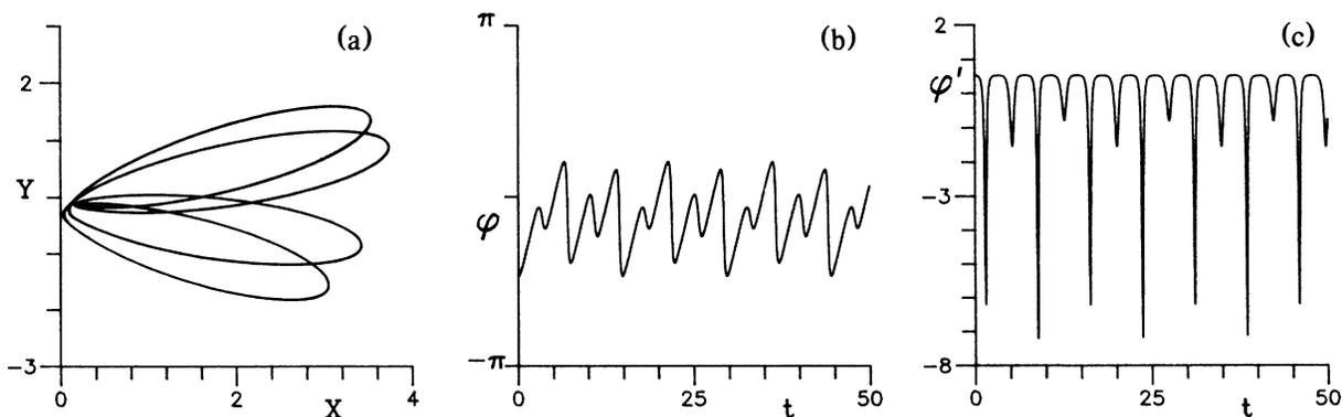
FIG. 4. For the same parameters as in Fig. 3, solutions of Eqs. (1) after subtracting from the electric field phase the contribution  $0.48\gamma_{\perp}t$  which defines a new rotating frame; (a) imaginary vs real part of the electric field; (b) phase of the field; (c) instantaneous field frequency.
