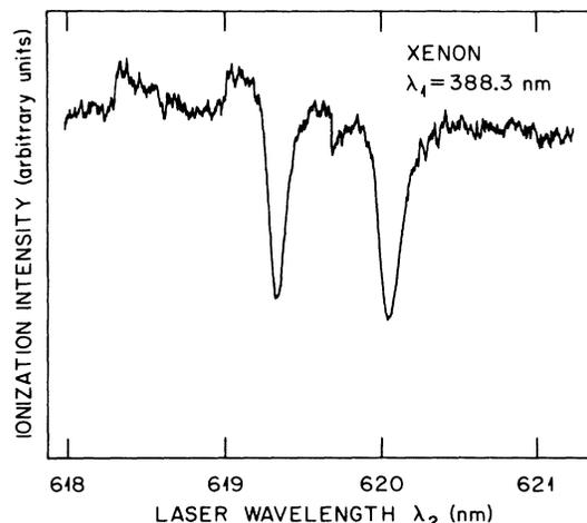
FIG. 8. Xenon  $5f$  resonances from 25 Torr of xenon in 150 Torr of argon. Laser one is fixed to a wavelength where dips occur as in the previous figure, and laser two is scanned.
