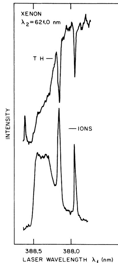
FIG. 6. Scan of laser one over the xenon  $6s'$  region while laser two excites transitions to the  $5f$  states. The top trace shows third-harmonic yield and the bottom, ion yield. The xenon pressure is 10 Torr.
