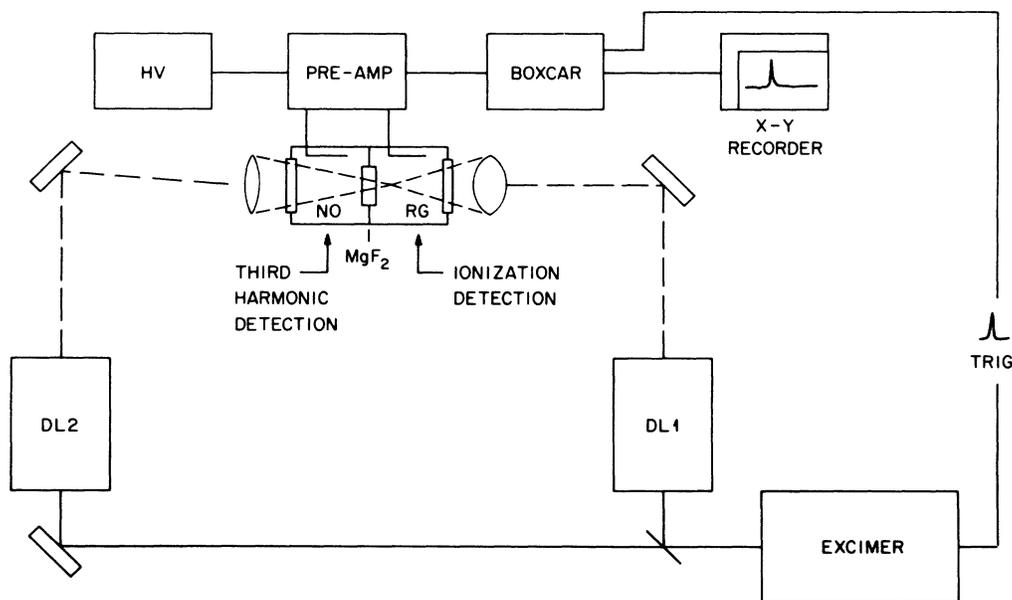
FIG. 1. Schematic diagram of the apparatus used to detect two-color MPI and THG. The output of an excimer laser is split and used to pump two dye lasers, DL1 and DL2. The two dye-laser outputs are focused into a rare-gas cell with a biased wire to collect electrons. A second such cell attached to the first via a common MgF<sub>2</sub> window allows third-harmonic detection from the photoionization of nitric oxide.
