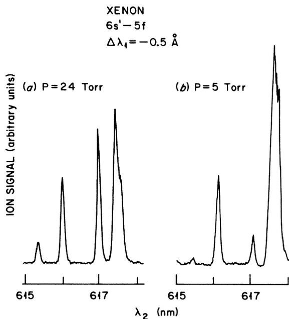
FIG. 10. Two-color scans over the xenon  $5f$  levels with laser one detuned  $0.5 \text{ \AA}$  to the red of the  $6s'$  level. Only the xenon pressure has been changed from (a) to (b). Marked differences in the relative intensities of the peaks are seen.
