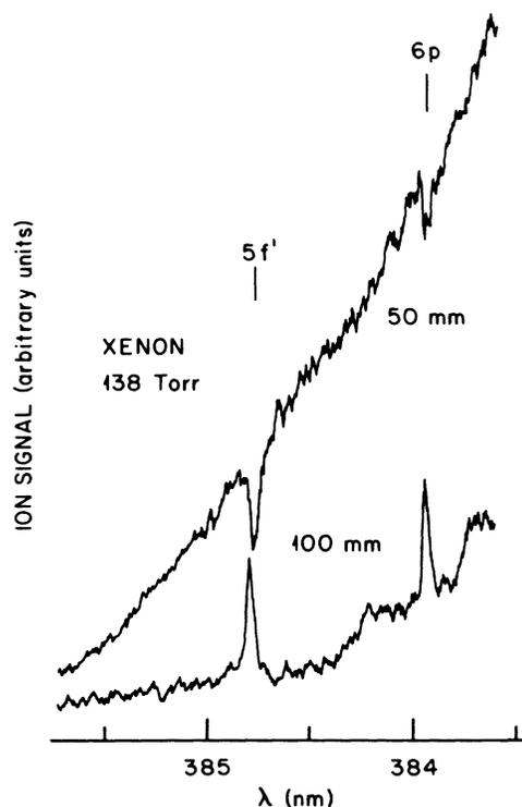
FIG. 9. “Accidental” (one-laser) excitation of the xenon  $5f'$  and  $6p$  states. The use of a shorter focal length lens causes the resonances to turn to dips.
