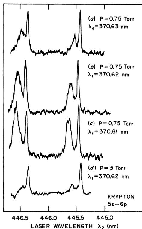
FIG. 3. Two-color excitation of the krypton  $6p$  resonances. The first laser is detuned to the blue of the  $5s$  state as in Fig. 2, while the second laser is scanned over the  $6p \left[ \frac{3}{2} \right]_1$  and  $6p \left[ \frac{3}{2} \right]_2$  states. Spectra (a)–(c) are from progressive detunings to the blue of the  $5s$  state, while (d) is for the same detuning as in (b) but at higher pressure.
