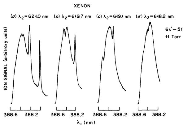
FIG. 7. Ionization spectra showing excitation of the  $5f$  states by third-harmonic light from the blue of the  $6s'$  state. Spectra (a)–(d) are obtained by setting laser two to progressively shorter wavelengths so that the  $5f$  resonances are excited progressively closer to the  $6s'$  state. When the resonances are “moved in” over the maximum of THG, they turn from peaks to dips in the ionization.
