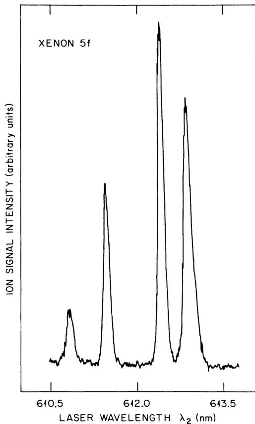
FIG. 5. Xenon  $5f$  levels excited by a scheme as shown in Fig. 2, with laser one detuned to the red of the xenon  $6s'$  level. The peaks, from left to right, are the  $5f[\frac{7}{2}]_4$ ,  $5f[\frac{5}{2}]_2$ ,  $5f[\frac{9}{2}]_4$ , and the  $5f[\frac{3}{2}]_2$  resonances. The pressure is 24 Torr.
