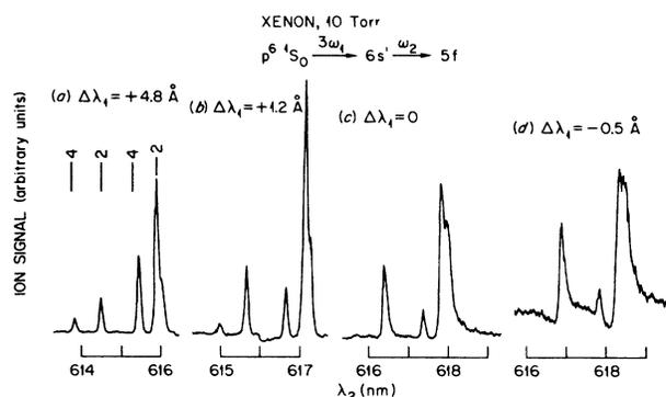
FIG. 11. Series of laser-two scans over the xenon  $5f$  levels excited near  $6s'-5f$  double resonances. Detuning of the first laser from the red of the  $6s'$  state over to the blue yields a smooth, continuous change in the appearance of the spectrum. Here we define  $\Delta\lambda_1$  as positive for a detuning to the red of the  $6s'$  state
