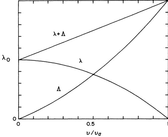
FIG. 4. Relative magnitudes of the NLS soliton width  $\lambda$  and the width  $\Lambda$  of the space-time shadow which contributes the speed dependence of the nonlinearity.
