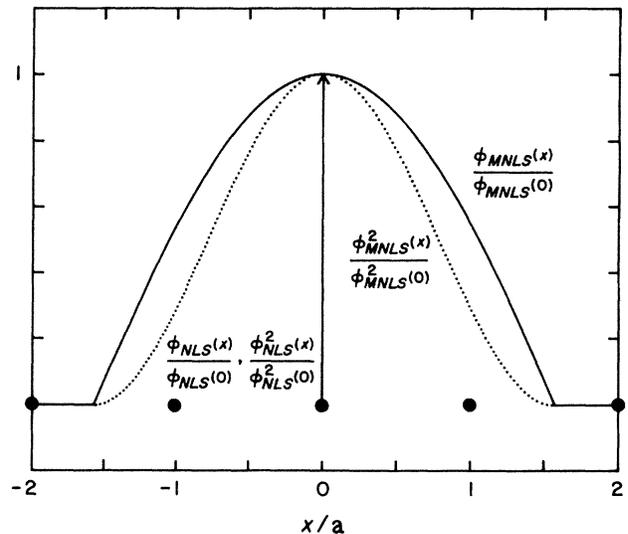
FIG. 6. Solid line (—), MNLS soliton envelope  $\phi_{MNLS}(x)/\phi_{MNLS}(0)$  in the high- $D$  limit; dotted line (⋯), MNLS probability density  $\phi_{MNLS}^2(x)/\phi_{MNLS}^2(0)$  in the high- $D$  limit. The corresponding NLS functions are singular distributions of vanishing width. (●) indicate lattice sites.
