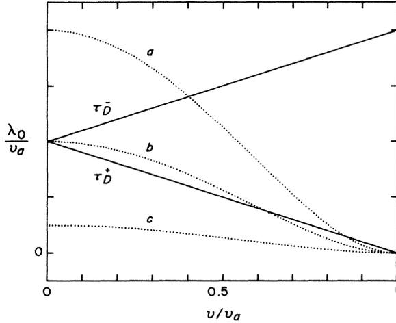
FIG. 2. Time scales for soliton formation. Solid lines (—), time scales for forward ( $\tau_D^-$ ) and backward ( $\tau_D^+$ ) propagating deformations to leave the excitation region; dotted lines ( $\cdots$ ), time scales for wave packet response ( $\tau_U$ ). Curve *a*,  $G_0/\hbar v_a < 1$ ; curve *b*,  $G_0/\hbar v_a = 1$ ; curve *c*,  $G_0/\hbar v_a > 1$ .
