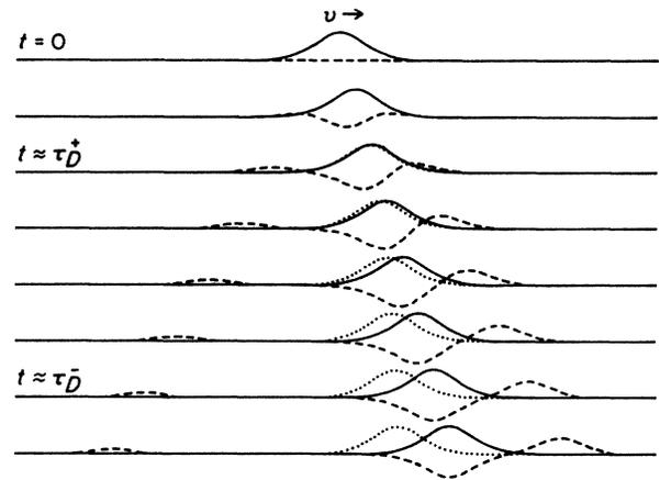
FIG. 1. Soliton formation. Solid lines (—), envelope of an initial wave packet, assumed to propagate as  $\rho(x-vt)$ ; dashed lines (---), potential  $U(x,t)$  in arbitrary units; dotted lines ( $\cdots$ ), hypothetical response of a wave packet when  $G_0/\hbar v_a > 1$ , based on the conclusions of Sec. IV A; the corresponding lattice response is not shown.
