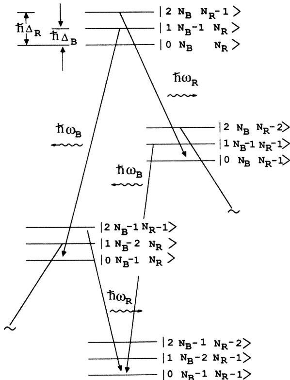
FIG. 2. Schematic energy levels of the eigenstates of the combined atom-field Hamiltonian which does not include laser-atom interactions. If the laser-atom interaction is included the states will still be grouped in three-state manifolds, but the energy splitting between states will be altered, and spontaneous decays will be allowed from all states.
