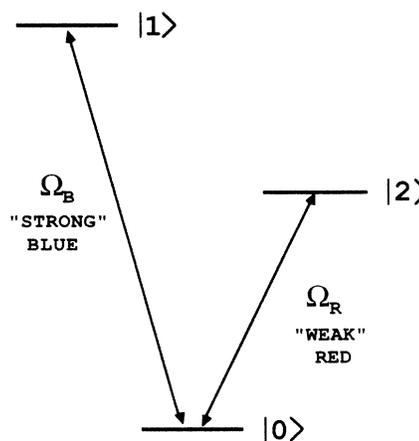
FIG. 1. "V" configuration for a single-atom quantum-jump experiment. The labeled states are eigenstates of the atomic Hamiltonian alone. The 0-1 transition is "strong" and the 0-2 transition is "weak." The 0-1 transition will be referred to as blue and the 0-2 transition as red.
