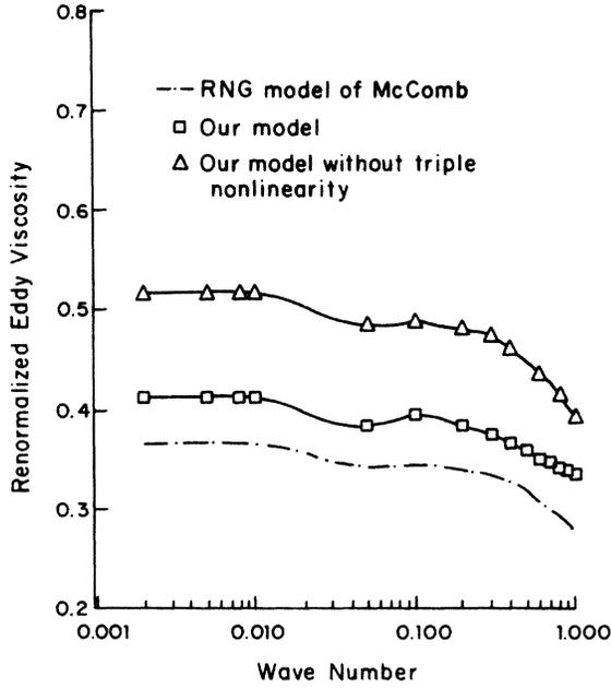
FIG. 2. Scaled renormalized eddy viscosity for a coarser subgrid partition ( $f=0.6$ ) chosen so that now only one memory term (arising from the triple nonlinearity) contributes to  $v^*$ . There is no cusp behavior exhibited—curves are labeled as in Fig. 1.
