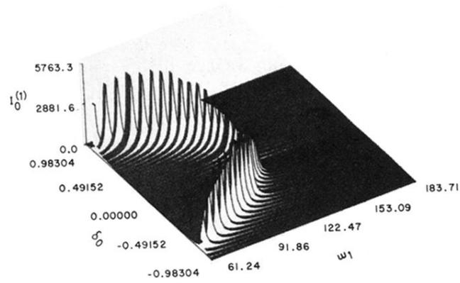
FIG. 1. Dependence of  $I_0^{(1)}$  on detuning  $\delta_0$  and  $\omega_1$  in case of frequency modulation. Excitation ration  $\varepsilon=2$  and  $k_0=1.5 \times 10^4$ .
