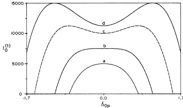
FIG. 3. Dependence of  $I_0^{(1)}$  on detuning  $\delta_{0p}$  ( $\omega_1 = \Omega$ ) for various values of  $\varepsilon$  in case of loss modulation.  $k_0 = 1.5 \times 10^4$  and (a)  $\varepsilon = 1.5$ , (b)  $\varepsilon = 2.0$ , (c)  $\varepsilon = 3.0$ , and (d)  $\varepsilon = 4.0$ , respectively.
