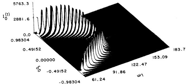
FIG. 1. Dependence of  $I_0^{(1)}$  on detuning  $\delta_0$  and  $\omega_1$  in case of frequency modulation. Excitation ratio  $\varepsilon=2$  and  $k_0=1.5 \times 10^4$ .
