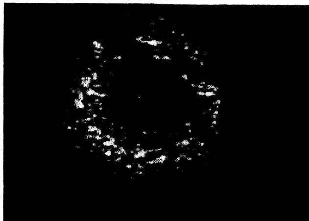
FIG. 5. Typical spinodal decomposition ring obtained by light scattering 70 s after the beginning of the quench ( T_c - T_f = 3 \text{ mK} , K_m = 3.8 \times 10^3 \text{ cm}^{-1} , C^*C\text{-M} system).
