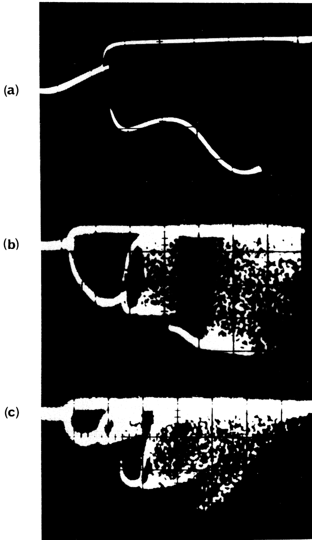
FIG. 9. Influence of the laser frequency on the BD obtained with the modulation amplitude as a control parameter in conditions of relatively low laser gain. The cavity detuning is, respectively, (a) 0, (b) 25, (c) 100 Mhz.
