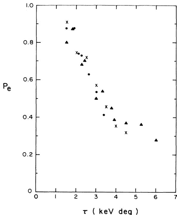
FIG. 4. The probability of electronically elastic scattering in the direct channel  $P_e$  as a function of  $\tau$  for beam energies of 1.5 keV (●), 2.0 keV (×), and 3.0 keV (▲).
