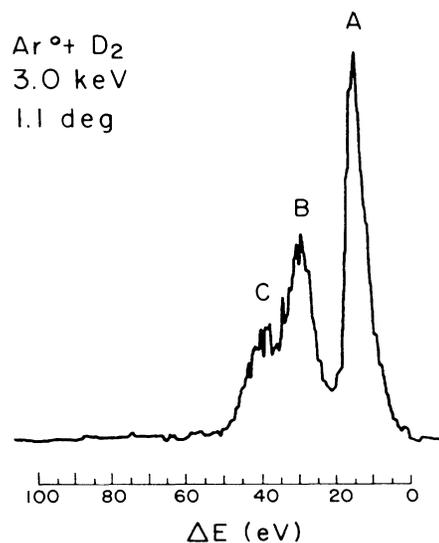
FIG. 1. Energy spectrum of the direct scattering of Ar by D<sub>2</sub>. The 3-keV Ar projectile is scattered through a laboratory angle of 1.1°.
