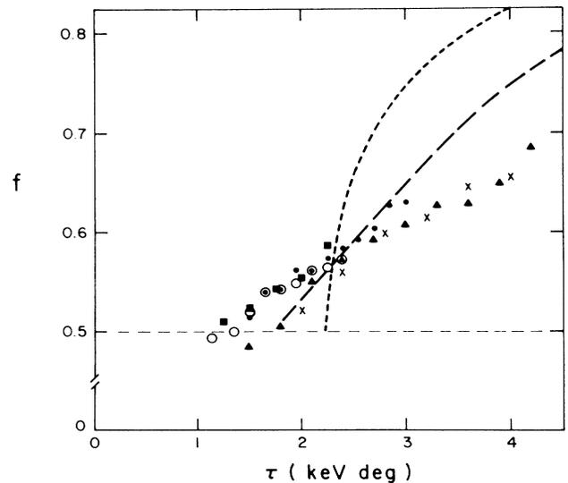
FIG. 3. Energy loss  $f(\tau)$  at five different beam energies: 750 eV ( $\circ$ ), 1.0 keV ( $\blacksquare$ ), 1.5 keV ( $\bullet$ ), 2.0 keV ( $\times$ ), and 3.0 keV ( $\blacktriangle$ ). All  $f$  values were reduced using the full Eq. (3) for  $\Delta E_{\text{elas}}$ . Results from two earlier experiments are superimposed on the plot: Ne + D<sub>2</sub> (long-dash curve) and He + D<sub>2</sub> (short-dash curve).
