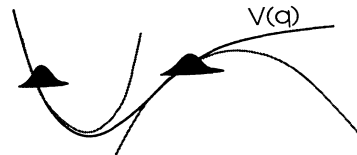
FIG. 2. A potential V(q) is approximated by a quadratic fit in the vicinity of the current position of the wave packet.
