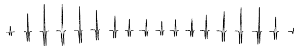
FIG. 6. The raw spectroscopic data showing the center depletion. The absorption line is the P (3) transition of ArH + fundamental band. The detection of the spectra was made by frequency modulation and 2 f detection. The signal-to-noise ratio is typically 100. The spatial separation between adjacent signals is approximately 1 mm.
