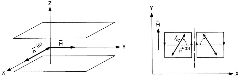
FIG. 1. Schematic representation of the geometry of the nematic sample. Flows generated by oppositely rotating zones which explain the appearance of transient structures are also schematically displayed.
