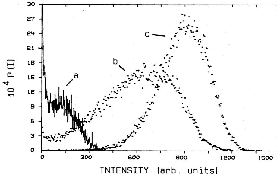
FIG. 1. Normalized distributions of the experimental laser intensity  $P(I)$  taken at three different laser working points. Curve  $a$ ,  $\langle I \rangle = 32$ . The initial point of the distribution,  $P(0)$ , is approximately 50. Curve  $b$ ,  $\langle I \rangle = 590$ . The initial point of the distribution,  $P(0)$ , is approximately 0.54. Curve  $c$ ,  $\langle I \rangle = 890$ ,  $P(0) \approx 0$ . Intensities are given in arbitrary units.
