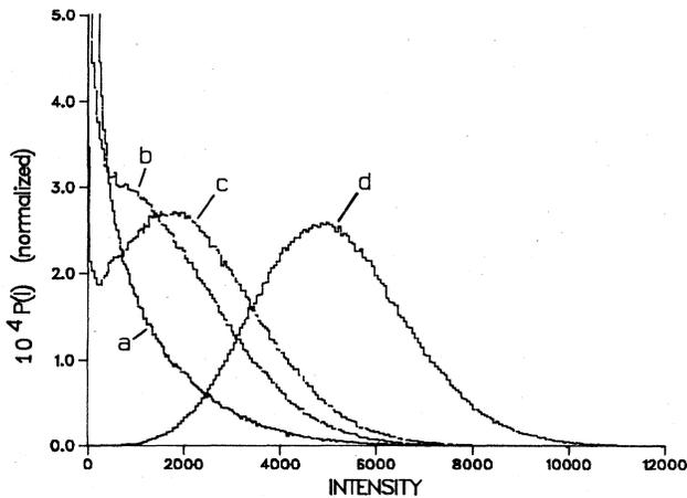
FIG. 3. Distributions of laser intensity  $P(I)$  as extracted from simulations of Eqs. (1)-(3), taken with four different average pump parameters: curve *a*,  $a = 400$ , curve *b*,  $a = 1000$ , curve *c*,  $a = 2100$ , and curve *d*,  $a = 5000$ . The noise parameters were fixed at  $Q = 5000$  and  $\Gamma = 1000$ .
