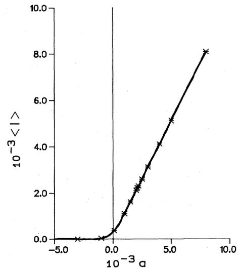
FIG. 5. Plot of the mean intensity vs the true control parameter, the pump parameter  $a$ . The noise parameters were fixed at  $Q = 5000$  and  $\Gamma = 1000$ .
