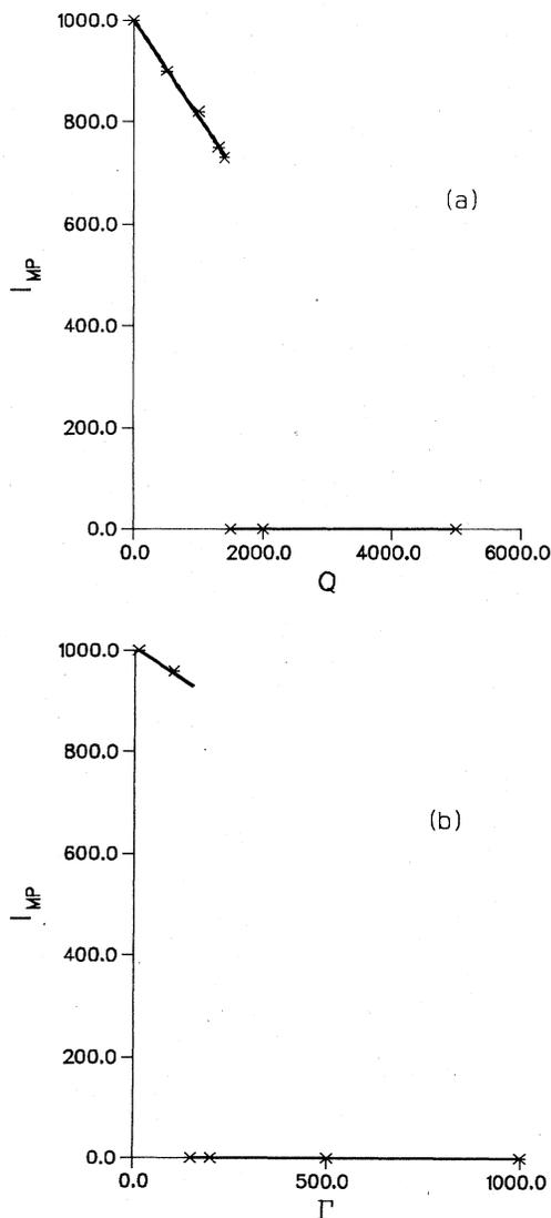
FIG. 6. (a) Plot of the most probable intensity vs the noise strength  $Q$ . The other parameters were fixed at  $a=1000$  and  $\Gamma=1000$ . (b) Plot of the most probable intensity vs the noise bandwidth  $\Gamma$ . The other parameters were fixed at  $a=1000$  and  $Q=5000$ .
