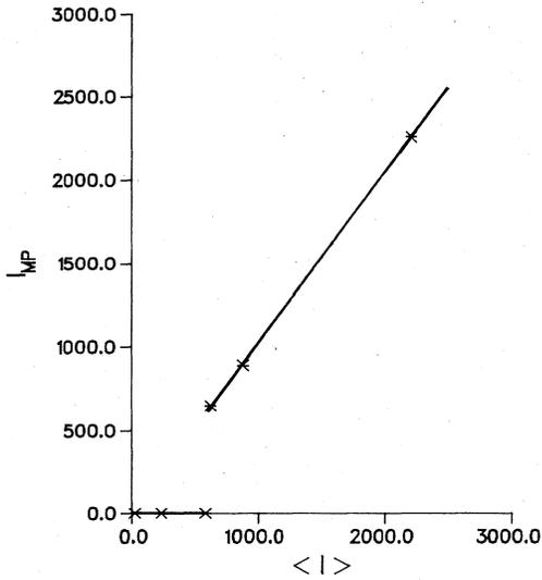
FIG. 2. Plot of the experimentally determined most probable intensity vs the mean intensity of the dye laser showing the first-order phase-transition analogy.
