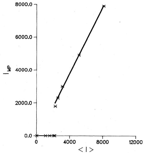
FIG. 4. Plot of the most probable intensity vs the mean intensity taken from simulations of Eqs. (1)-(3). The noise parameters were fixed at  $Q = 5000$  and  $\Gamma = 1000$ .
