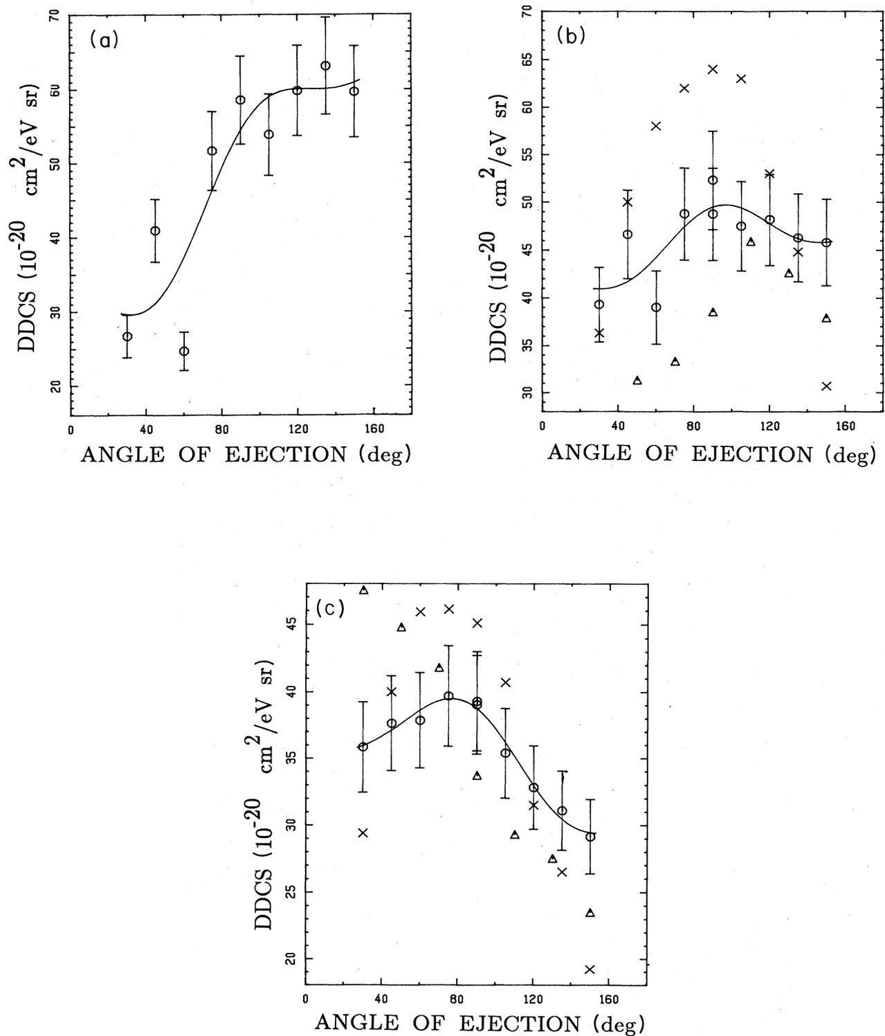
FIG. 5. Absolute DDCS for  $N_2$  at a primary energy of 500 eV. The circles denote the present measurement. The triangles represent the results of DuBois and Rudd; the  $\times$ 's represent the results of OBP; the solid line is a fit to an expansion in Legendre polynomials using the present data. The measurements at 2, 4, 10, 20, and 40 eV ejected energy are designated by *a, b, . . . , e*, respectively.
