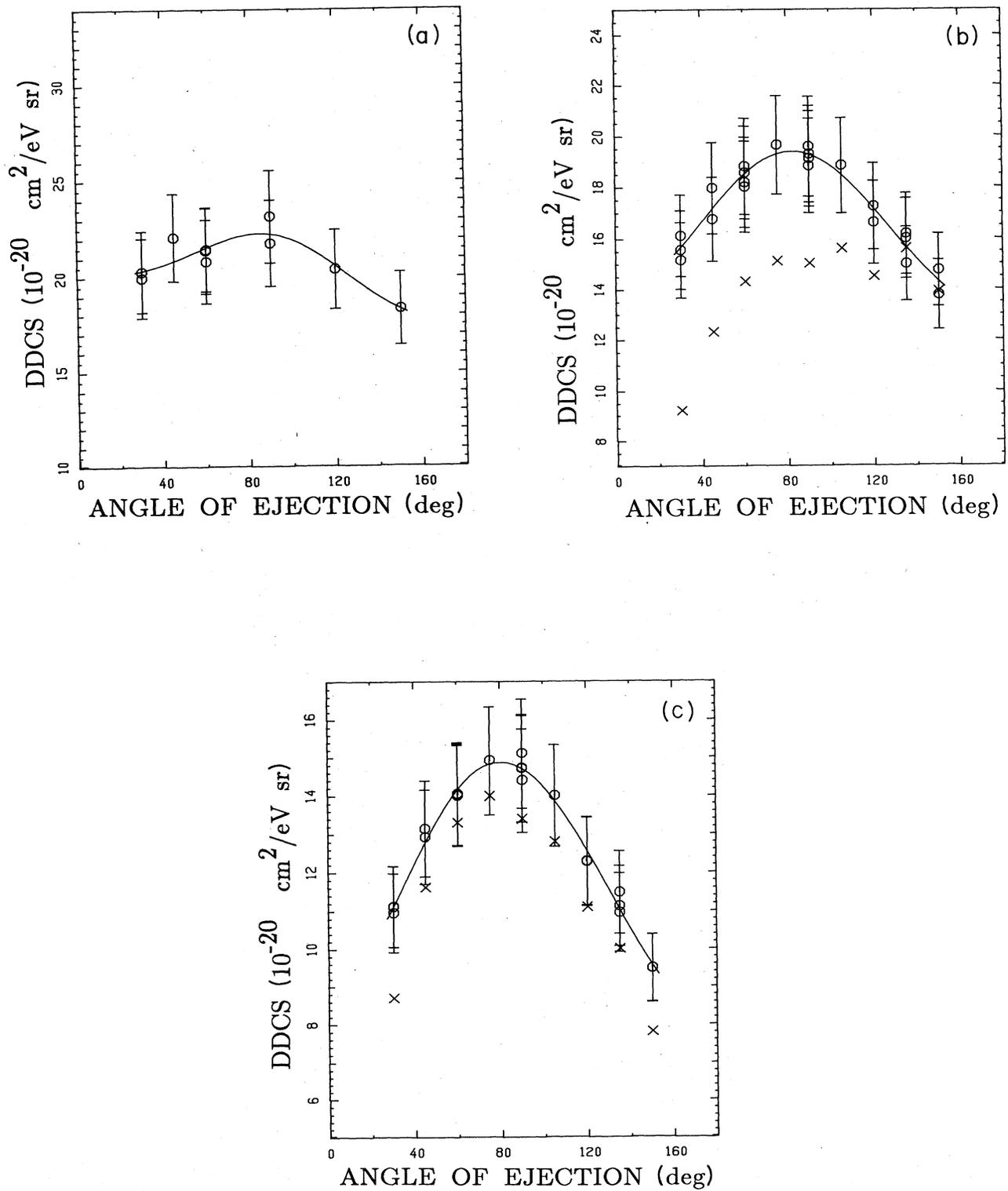
FIG. 7. Absolute DDCS for  $N_2$  at a primary energy of 2000 eV. The circles denote the present measurement. The  $\times$ 's represent the results of OBP, the solid line is a fit to an expansion in Legendre polynomials using the present data. The measurements at 2, 4, 10, 20, and 40 eV ejected energy are designated by *a*, *b*, ..., *e*, respectively.
