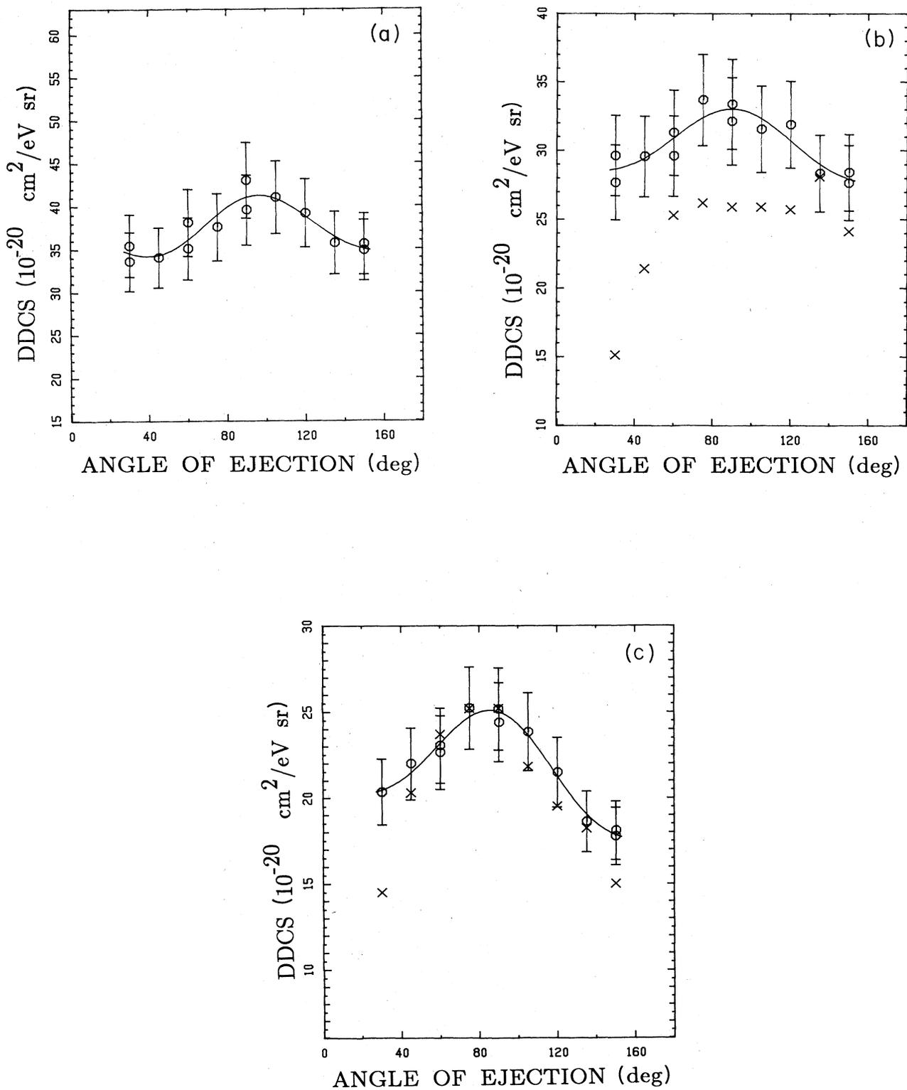
FIG. 6. Absolute DDCS for  $N_2$  at a primary energy of 1000 eV. The circles denote the present measurement. The  $\times$ 's represent the results of OBP, the solid line is a fit to an expansion in Legendre polynomials using the present data. The measurements at 2, 4, 10, 20, and 40 eV ejected energy are designated by *a, b, . . . , e*, respectively.
