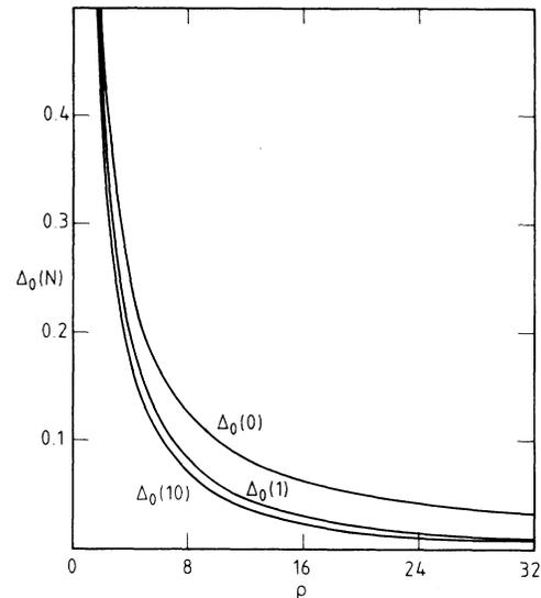
FIG. 4. Adiabatic effective potentials  $\Delta_0(N)$ , derived from  $(2N+1)$  coupled equations, as functions of the hyperradius  $\rho$  for the repulsive case  $c=1$ . On the scale of the graph,  $\Delta_0(\infty)$  is indistinguishable from  $\Delta_0(10)$ .
