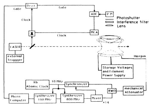
FIG. 2. Experimental setup for the laser-microwave double resonance experiment on <sup>173</sup>Yb<sup>+</sup>.
