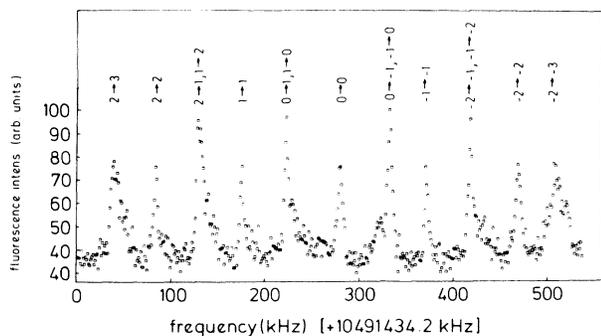
FIG. 3. Ground-state hyperfine Zeeman spectrum of  $^{173}\text{Yb}^+$  at  $B = 10^{-5}$  T. The numbers  $(i, j)$  at each line correspond to the initial  $(i)$  and final  $(j)$   $m_F$  state of the  $F = 3 - F = 2$  transition.
