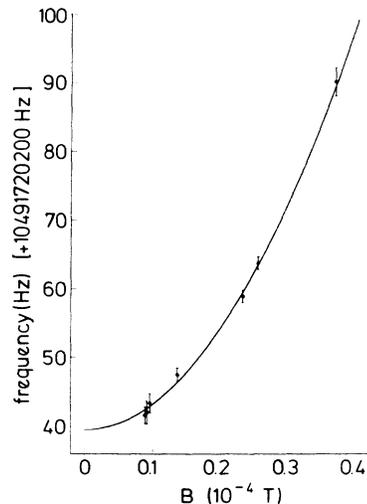
FIG. 5. Magnetic field dependence of the  $F = 3, m = 0 - F = 2, m = 0$  hyperfine transition. Fit according to the Breit-Rabi formula to the experimental points.
