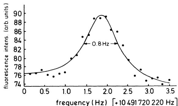
FIG. 4. Magnetic field "independent"  $F = 3, m = 0 - F = 2, m = 0$  transition. The solid line corresponds to a Lorentzian line shape and a linear decreasing background.
