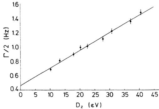
FIG. 7.  $|3,0\rangle$ - $|2,0\rangle$  linewidth [full width at half maximum (FWHM)] vs trap potential depth.
