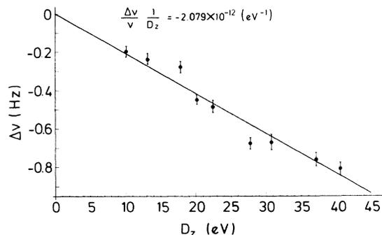
FIG. 6.  $|3, 0\rangle - |2, 0\rangle$  resonance frequency vs average trap potential depth for spherical potential shape.
