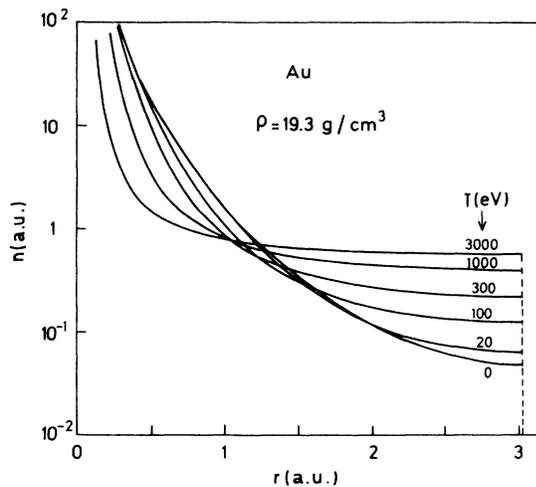
FIG. 1. Profiles of electron densities (in atomic units) for gold atoms confined within a spherical cell of radius  $r_0 = 3.02 \text{ a.u.}$  (this corresponds to the normal density,  $\rho = 19.3 \text{ g/cm}^3$ ). Calculations are shown for temperatures  $T = 0, 20, 100, 300, 1000,$  and  $3000 \text{ eV}$ .
