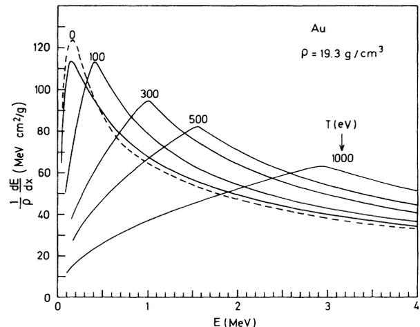
FIG. 2. Stopping power of confined gold atoms, according to the model described in the text, for temperatures  $T = 0, 100, 300, 500,$  and  $1000 \text{ eV}$ , versus proton energy. The dashed line indicates the experimental values for cold targets.
