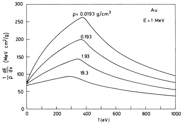
FIG. 3. Density and temperature dependence of the stopping power, for 1-MeV proton beams in gold. The enhancement of the energy loss becomes greater at lower densities, due to a larger relaxation of quantum constraints (see the text for discussion).
