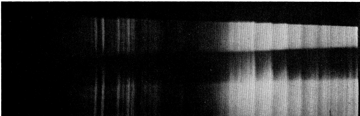
FIG. 3. Spatially resolved x-ray spectrum of a laser-produced praseodymium plasma.
