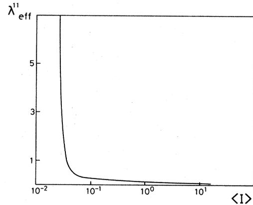
FIG. 6.  $\lambda_{\text{eff}}^{11}$  vs  $\langle I \rangle = \langle I_1 \rangle + \langle I_2 \rangle$  for a two-mode laser,  $\xi = 2$ ,  $\Delta a = 0$  including pumping fluctuations.  $\lambda_{11}(0)$  obtained from simulation with  $Q = 500$ ,  $\Gamma = 5$  (Ref. 27).
