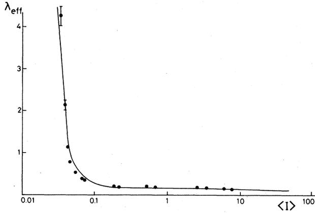
FIG. 1.  $\lambda_{\text{eff}}$  vs  $\langle I \rangle$  for a single-mode dye laser with pumping fluctuations. Intensity scale in arbitrary units. Continuous line follows from the simulation of (2.12) with  $Q=300$ ,  $\Gamma=5$  (Ref. 17). Dots follow from experimental results of Ref. 17.
