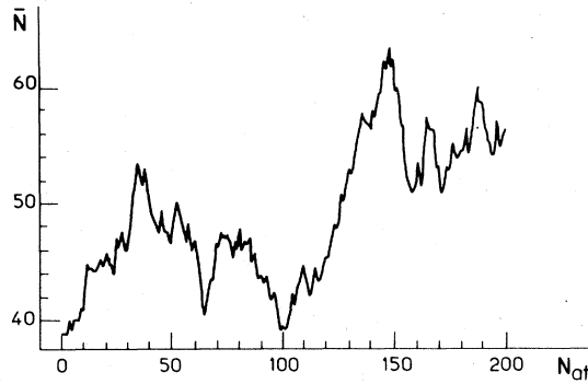
FIG. 8. Average photon number \bar{N}(N_{\text{at}}) for a two-photon micromaser with fluctuating t_{\text{int}} and t_{\text{at}} - t_{\text{int}} . Average values of t_{\text{int}} and t_{\text{at}} are the same as in Figs. 6 and 7. Mean-square-root deviations are \Delta t_{\text{int}} = 5.6 \times 10^{-3} t_{\text{cav}} , \Delta(t_{\text{at}} - t_{\text{int}}) = 1.1 \times 10^{-2} t_{\text{cav}} . Triggering field is the same as for Fig. 6.
