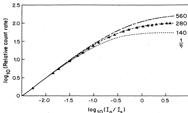
FIG. 3. Measured and calculated saturation curves with a long interaction region for the 5535-Å barium resonance. Reciprocal branching ratios of 140, 280, and 560 were assumed for the calculated curves and the saturation intensity  $I_s$  is 147  $\mu\text{W}/\text{mm}^2$ .
