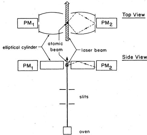
FIG. 2. Diagram of the atomic-beam chamber and light collector detector. Two orthogonal views are shown. The light collection efficiency is uniform over the laser-atomic-beam interaction region at the common line focus of the double elliptical cylinder.
