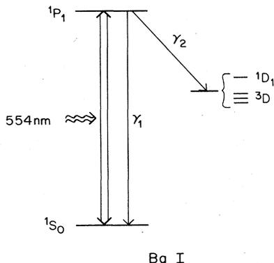
FIG. 1. Relevant energy levels in the Ba I spectrum. The  $D$ -state lifetimes are  $\approx 0.5$  sec (Ref. 13) and transitions back to the ground state play no role in the present experiments.
