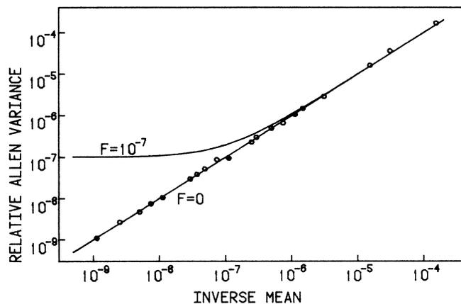
FIG. 1. Comparison of measured Allen variance with predictions of a simple process, and a compound process with a flicker floor of  $10^{-7}$ . The open circles correspond to data taken at a rate of  $6.4 \times 10^5 \text{ sec}^{-1}$ . For the closed circles, the rate was  $3 \times 10^6 \text{ sec}^{-1}$ .
