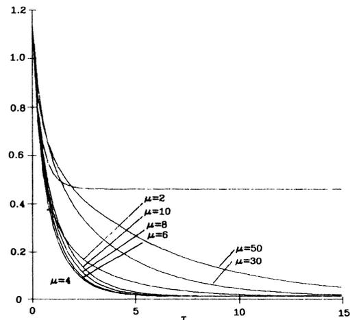
FIG. 5. The approach to thermal equilibrium of an equimolar mixture as described by  $H(\tau) - H_{eq}$  for  $c_1 = c_2$ . Both  $H(0) - H_{eq}$  and  $\dot{H}(0)$  are independent of the mass ratio  $\mu$ . Note the interesting dependence on the mass ratio, and especially, that for  $\mu = 1$  the system does not approach the same limit.
