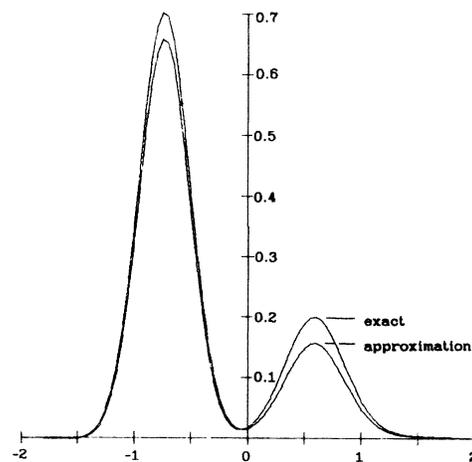
FIG. 2. For  $\tau = 0.5$ ,  $c_1 = c_2$ , and  $\mu = 1.5$  the exact solution for  $h_1(x, \tau)$  [see Eq. (51a)] is compared with the solution of the difference equation [Eq. (53a)]. The mean velocity of the second branch is determined by momentum and energy conservation in the first collision.
