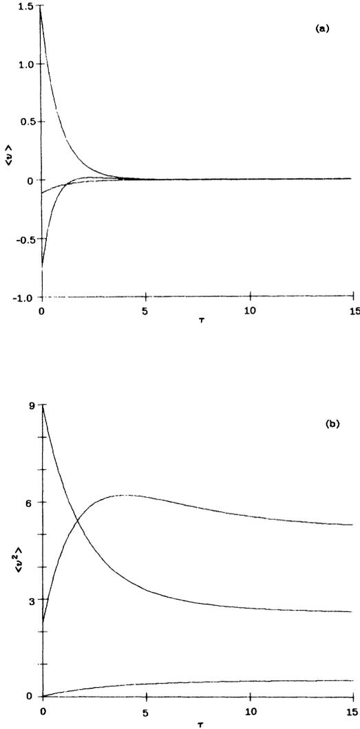
FIG. 6. For a ternary mixture with  $c_1=c_2=0.25$ ,  $c_3=0.5$ ,  $m_1:m_2:m_3=1:2:20$  and delta functions located at  $v_1^0=-3$ ,  $v_2^0=6$ ,  $v_3^0=-0.225$  as initial conditions, the time dependence of (a) the mean velocities and (b) the mean-square velocities is shown. Note, that for the lightest component the equilibrium value is not approached monotonically.
