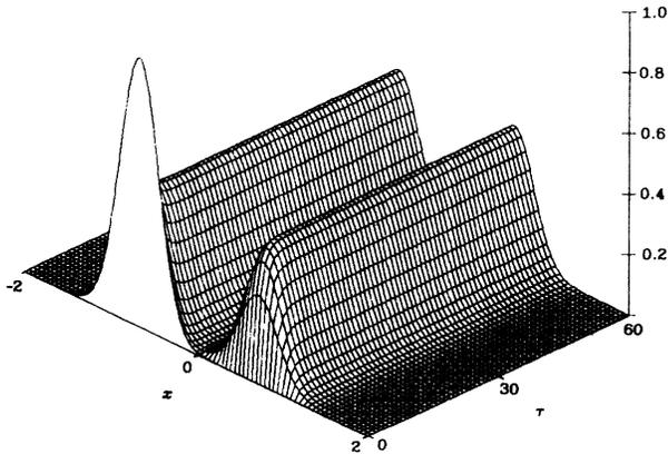
FIG. 4. The distribution of particles "1" of a binary mixture with  $\mu = 1$  and  $c_1 = c_2$ , where the initial distributions are at  $\pm v^0$ , respectively. From Eq. (7) it is known that the sum of the initial distributions does not change with time and does therefore not approach a Maxwell-Boltzmann distribution. The redistribution of velocities between the two components can be seen from the changes in the distribution of the particles "1" [cf. Eq. (8)].
