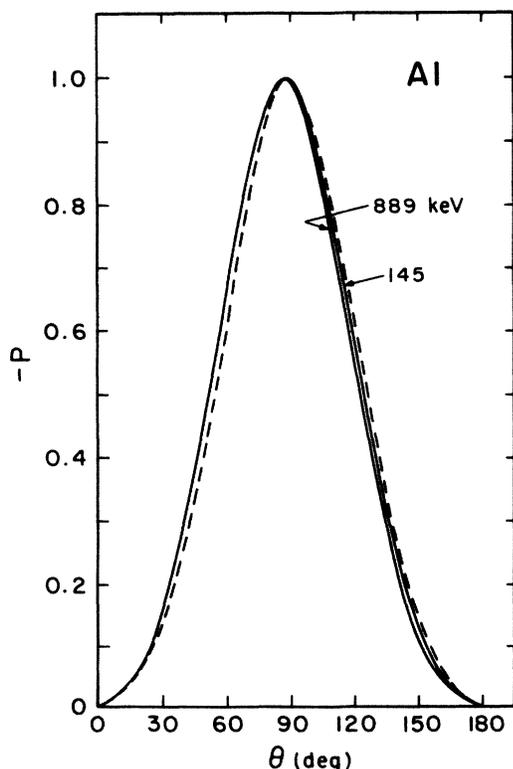
FIG. 2. Variation of polarization with scattering angle for photon energies 145 and 889 keV for aluminum ( $Z=13$ ), according to our calculations (solid curves). The dashed curve shows the energy-independent FF values.
