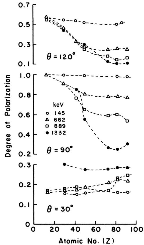
FIG. 5. Variation of polarization with atomic number ( $Z$ ) for different photon energies at three scattering angles.
