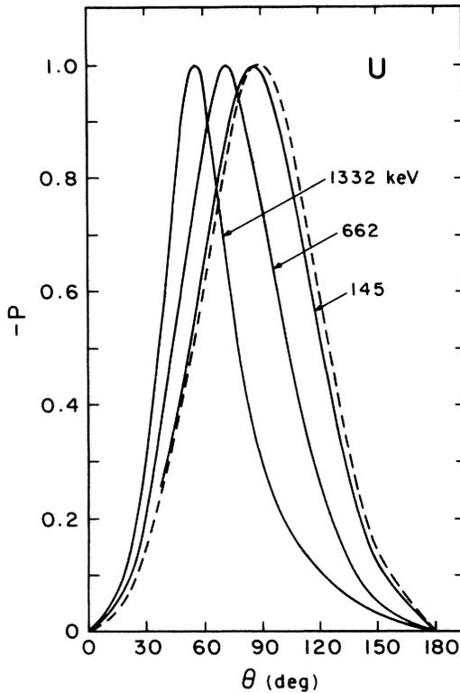
FIG. 4. Variation of polarization with scattering angle for uranium ( $Z=92$ ) at different photon energies, according to our calculations. The dashed curve shows the energy-independent FF values.
