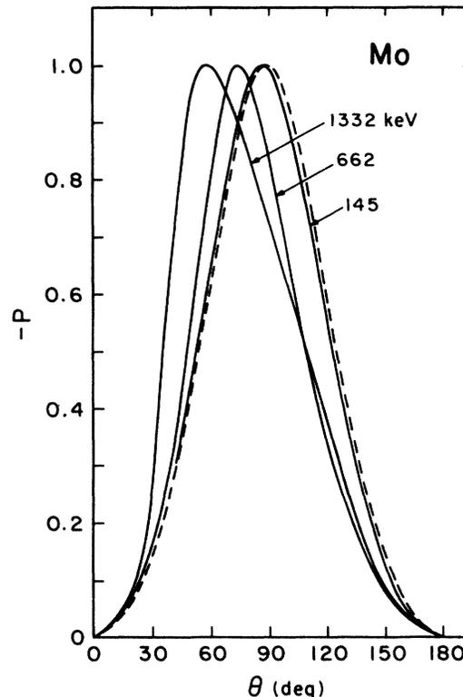
FIG. 3. Variation of polarization with scattering angle for molybdenum ( $Z=42$ ) at different photon energies, according to our calculations. The dashed curve again shows the energy-independent FF values.
