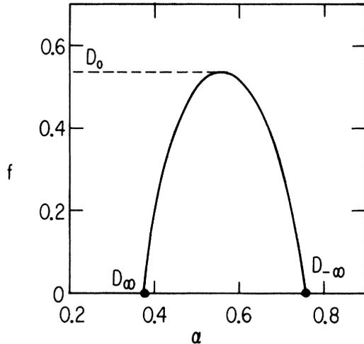
FIG. 1. The spectrum of scaling indices  $f(\alpha)$  found for the critical period-doubling attractor. The maximum point is the fractal dimension  $D_0$ , and  $\alpha_{\min} = D_\infty = \ln 2 / \ln \alpha_{PD} = 0.37775 \dots$  and  $\alpha_{\max} = D_{-\infty} = \ln 2 / \ln \alpha_{PD} = 0.75551 \dots$  (Ref. 2).
