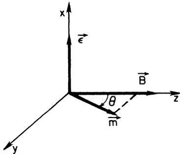
FIG. 2. Typical interaction region field configuration consisting of a static magnetic field  $\mathbf{B}$ , an oscillating electric field  $\epsilon(t) = \epsilon \cos(\nu t)$ , and an oscillating magnetic field  $\mathbf{m}(t) = \mathbf{m} \cos(\nu t)$ .
