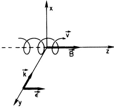
FIG. 10. Effect of a motional electric field is illustrated by considering an ion traveling in a helical motion along the static magnetic field. The ion passes through a beam of microwaves which is polarized along the static magnetic field.
