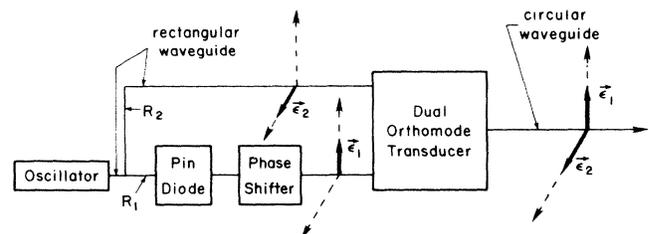
FIG. 7. Scheme allowing for complete control of the polarization of microwaves.
