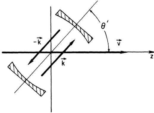
FIG. 6. Modes of a Fabry-Perot resonator can be expressed as a linear combination of two traveling waves. An ion traversing the resonator as shown will see two frequencies because of the Doppler effect. If the frequency separation is larger than the linewidth of the transition of interest, it is possible to separately resolve the two components. This provides a means for reversing the propagation vector  $\mathbf{k}$  by tuning the microwave frequency.
